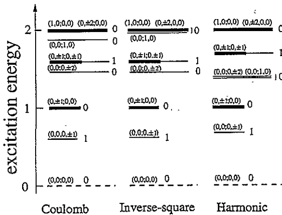
Figure 4. Theoretical energy-level spectrum for N = 2 electrons in a d = 2 dimensional parabolic quantum dot at zero magnetic field for various forms of the electron–electron interaction. Energies are shown in units of \hbar\omega_0 with respect to the ground state. Expressions for the harmonic and inverse-square interaction levels are obtained analytically. The Coulomb spectrum is adapted from the numerical results of [75]. Lengths of thick and thin lines represent the number of centre-of-mass and relative quanta respectively, as for figure 3. Total spin S is indicated to the right of each level. Labellings in parentheses (n', m'; n, m) denote centre-of-mass- and relative-mode quantum numbers for the purpose of comparison with the Coulomb result.
